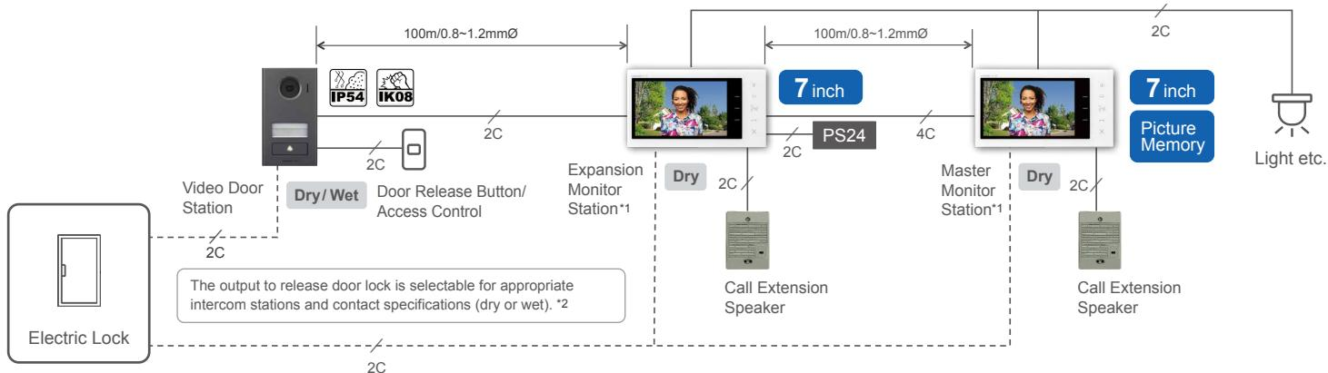
\*1. Room to room communication is not available. \*2. PT (AC transformer) is required when selecting dry contact.
